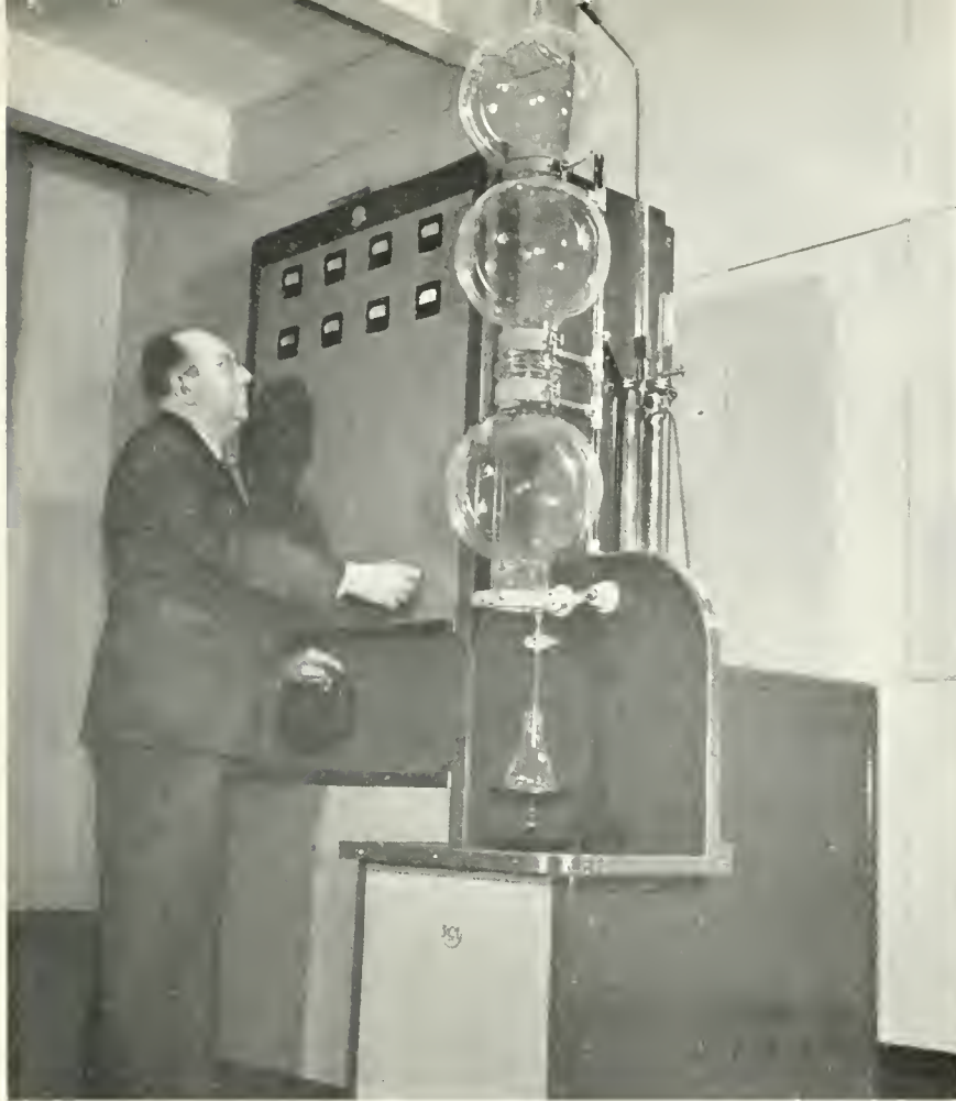
DR. GEORGE H. BROWN GIVES THE PENICILLIN ELECTRONIC DEHYDRATING APPARATUS HE DEVELOPED IN RCA LABORATORIES A FINAL INSPECTION BEFORE IT IS SHIPPED TO THE E. R. SQUIBB & SONS PLANT AT NEW BRUNSWICK, N. J.
